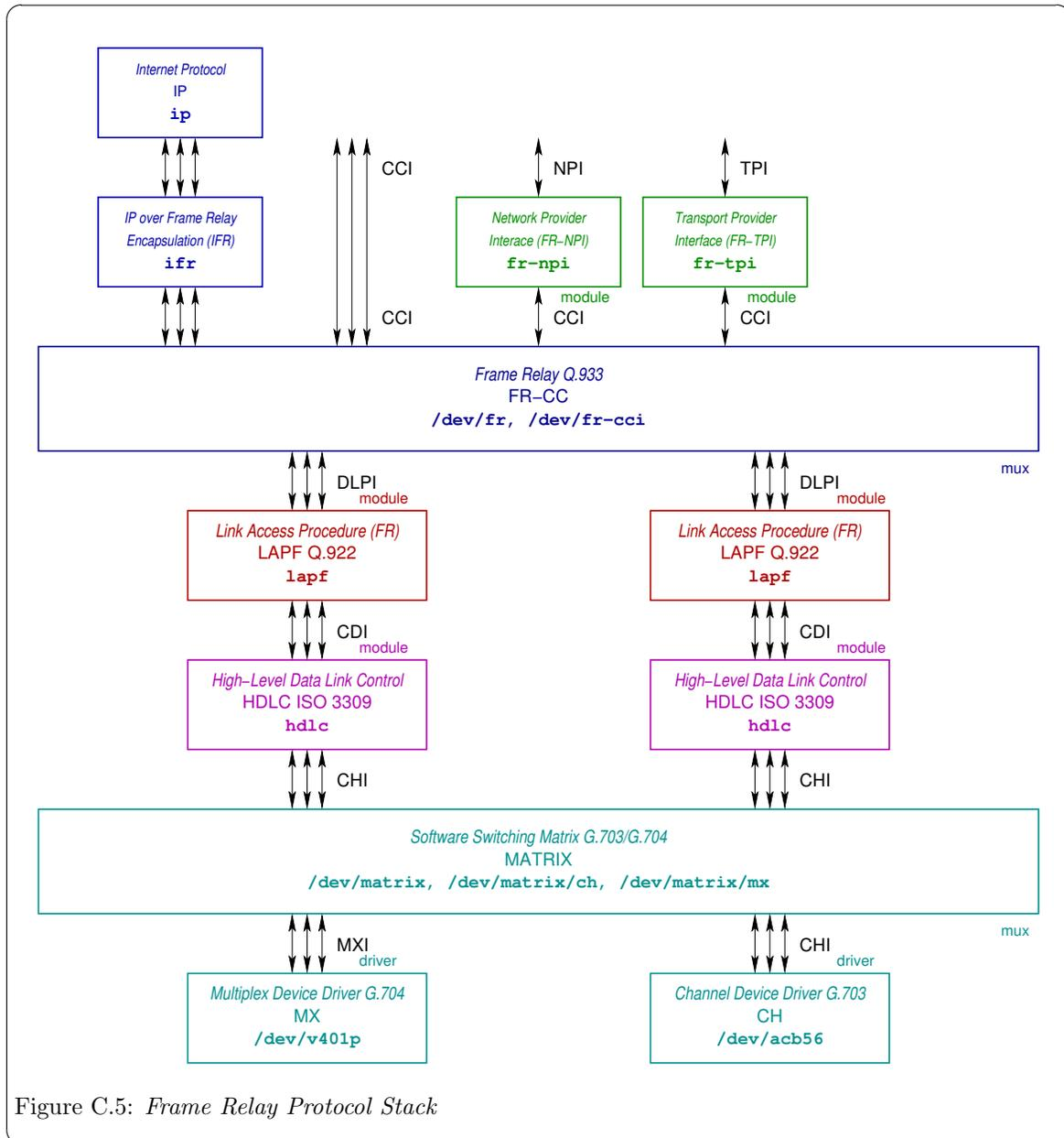
Figure C.5: Frame Relay Protocol Stack
