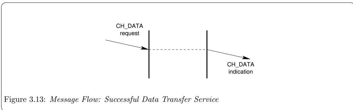
Figure 3.13: *Message Flow: Successful Data Transfer Service*
