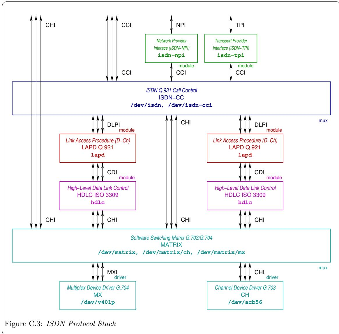
Figure C.3: ISDN Protocol Stack
