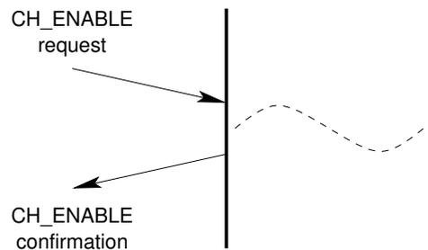
Figure 3.6: *Message Flow: Successful Enable Service*
