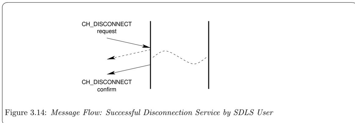
Figure 3.14: *Message Flow: Successful Disconnection Service by SDLS User*
