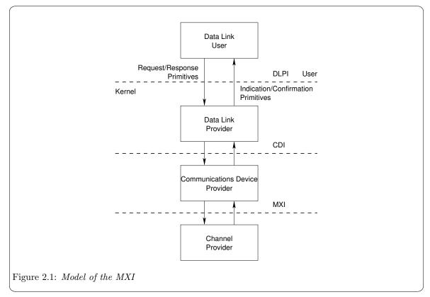
The MXI allows the MXS provider to be configured with any multiplex layer user (such as a signalling data terminal application) that also conforms to the MXI. A multiplex layer user can also be a user program that conforms to the MXI and accesses the MXS provider via **putmsg(2s)** and **getmsg(2s)** system calls. The typical configuration, however, is to place a signalling data terminal module above the multiplex layer.
