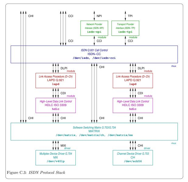
Figure C.3 illustrates the use of the MXI interface specification in the formation of the ISDN (Integrated Services Digital Network) protocol stack. The MXI interface provides two primary categories of access necessary for the ISDN protocol stack:
