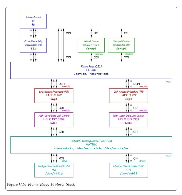
Use of the OpenSS7 softswitch matrix at the lowest level, as illustrated in Figure C.5, provides a mechanism whereby any available communications channel available to the host (including ISDN B-channels) can be used as a Frame Relay data link.
