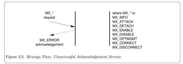
As illustrated in Figure 3.2, the service primitives for which a negative acknowledgement may be returned are the MX\_INFO\_REQ, MX\_ATTACH\_REQ, MX\_DETACH\_REQ, MX\_ENABLE\_REQ, MX\_DISABLE\_REQ and MX\_OPTMGMT\_REQ messages.
