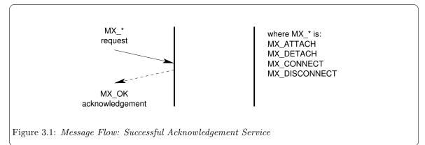
As illustrated in Figure 3.1, the service primitives for which a positive acknowledgement may be returned are the MX\_ATTACH\_REQ and MX\_DETACH\_REQ.
