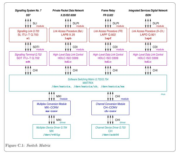
The MXI interface is responsible for providing access to communications channels (single-rate, multirate and full-rate) necessary for implementing the synchronous communications channels necessaary for implementing data communications links. Use of the *OpenSS7* software switch matrix at the
